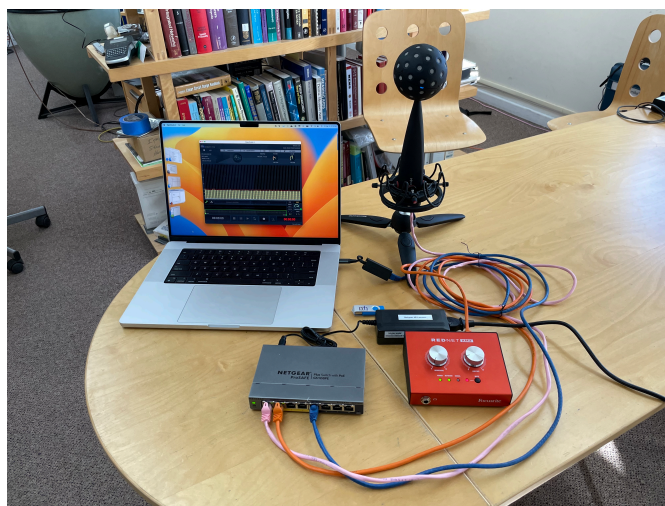
Figure 2: Photograph of the em64 array connected to a MacBook Pro with Gb ethernet dongle and running EigenStudio3. Picture also shows the Netgear GS108PEv3 PoE ethernet switch and RedNet AM2 Dante headphone amplifier.
